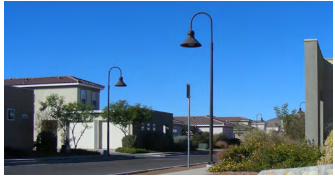
Downward-pointing, widely-spaced, energy-efficient street lamps can diminish light pollution.
