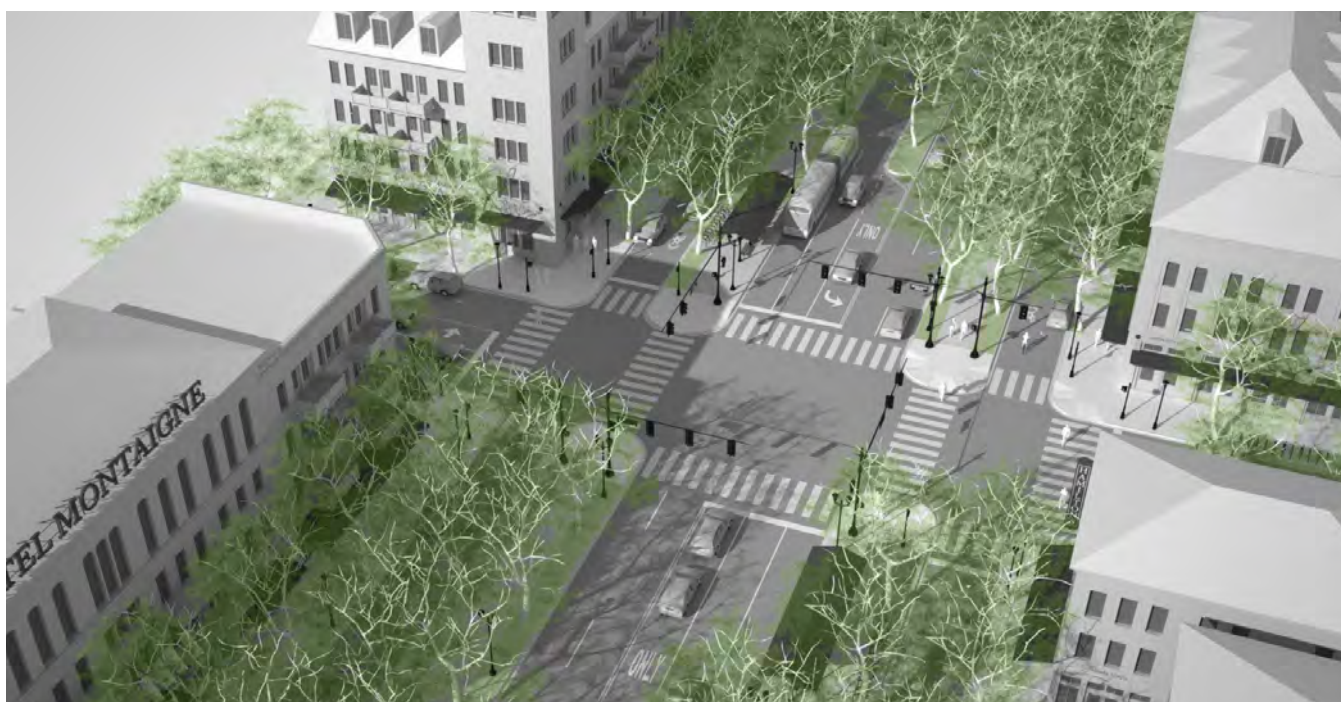
Multiway boulevards have center traffic lanes, and side traffic lanes that separate local and through traffic with tree-lined medians.
